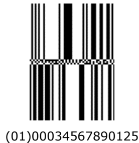
Abbildung 5.5.2.1.4-1. GS1 DataBar Stacked Omnidirectional
