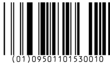
Abbildung 5.1.1-4. GS1 DataBar Omnidirectional Strichcode
